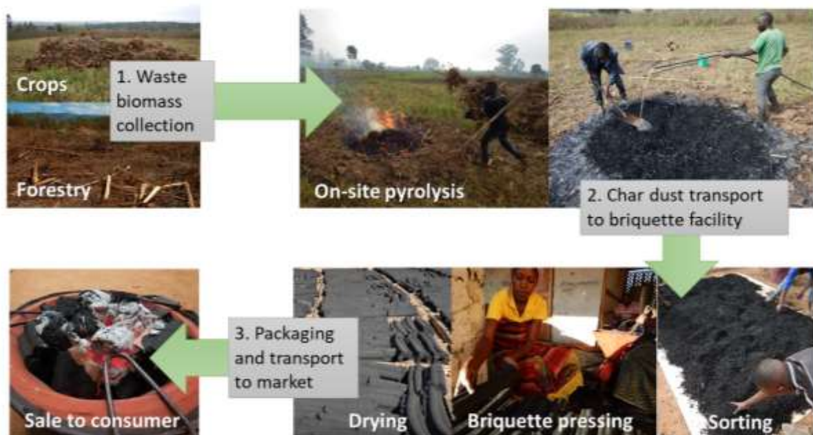
Figure 1. Overall concept behind the WBCBT project, showing how harvest waste biomass is converted to charcoal briquettes and sold to urban consumers for their cooking energy needs (thus substituting conventional wood-based charcoal)
