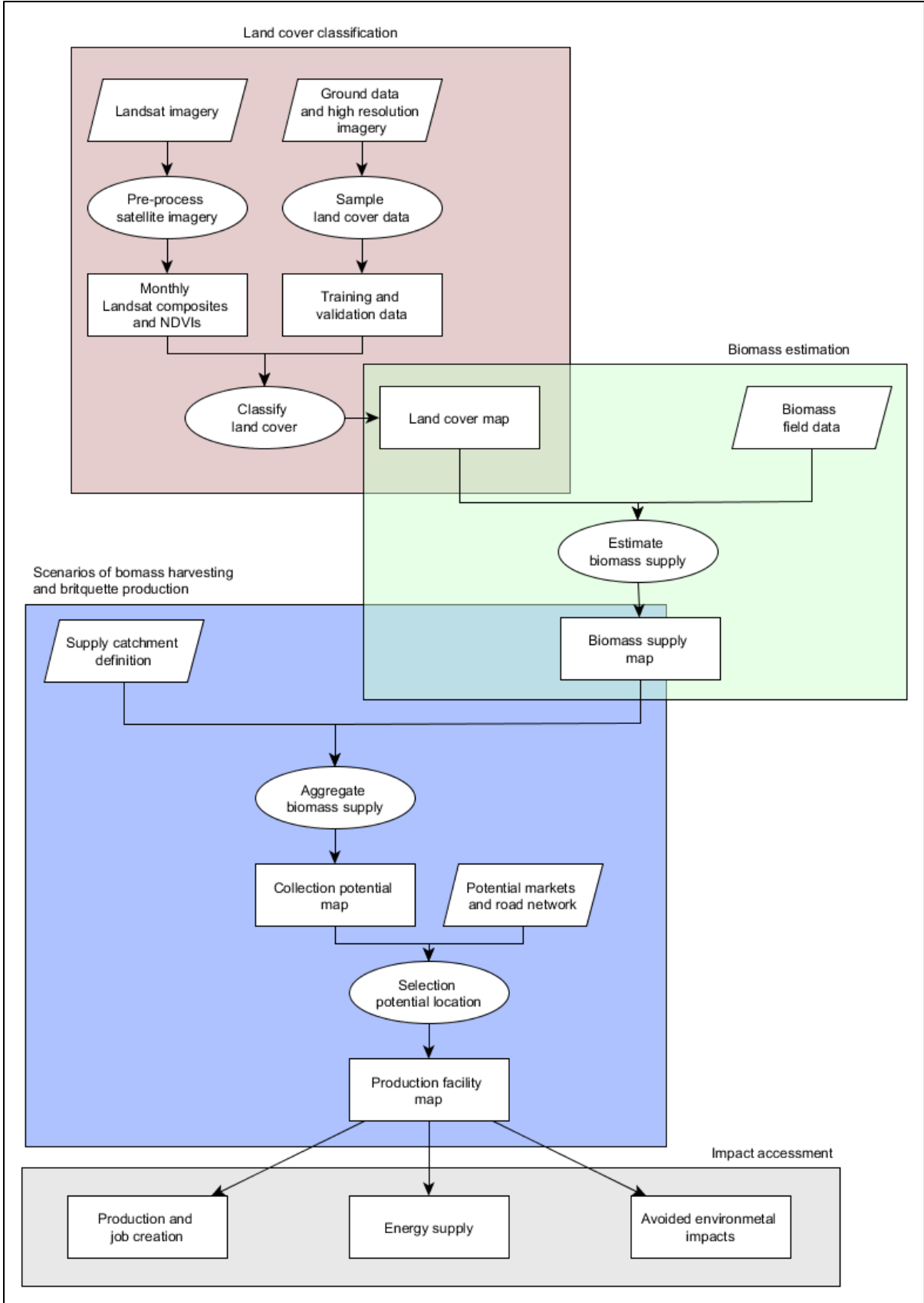
Figure 3: Overview of the modelling approach (parallelogram = input; oval = work step; rectangle = output)
