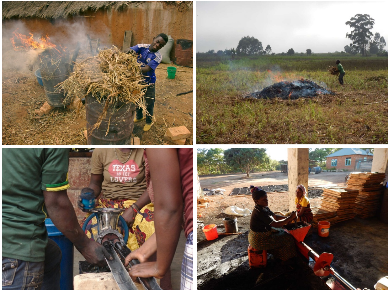
Figure 5-8: (top) A shift during project work from char dust production in portable kilns (left) to the flame curtain method (right); and (bottom) from the ARTI-supplied extruder to the EFCO-developed hydraulic extruder.
