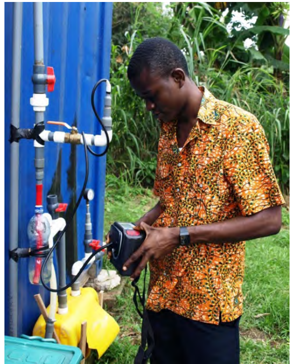
Figure 20: Gas measurement using Dräger X-am 7000
