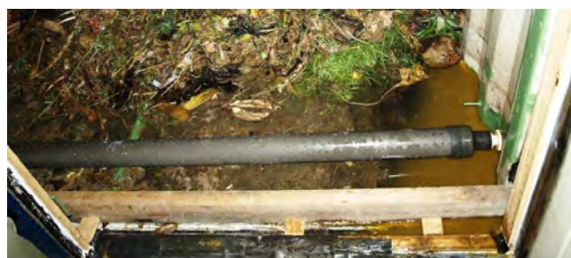
Figure 12: Loaded container after assembling the percolate outlet port
