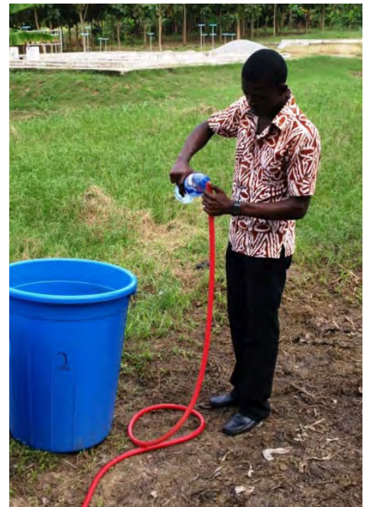
Figure 18: Filling the garden hose connected to the percolation system with water
