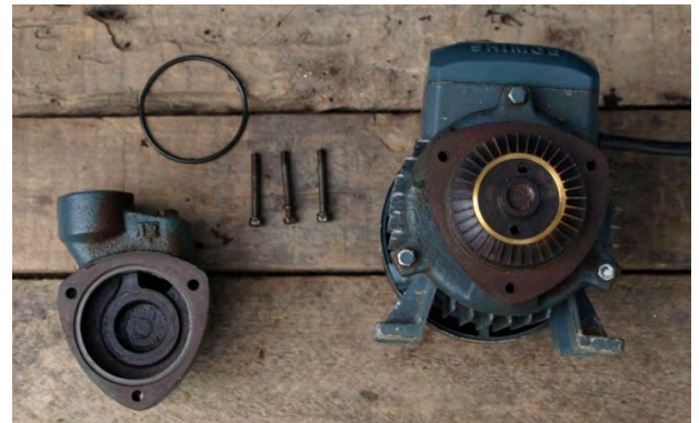
Figure 24: Percolation pump disassembled for cleaning
