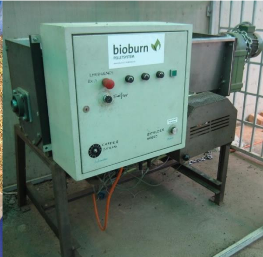
Figure 6: Bioburn pelletizer (Englund et al., 2016).
