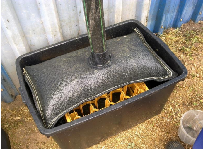
Figure 5: Bench-scale geotube for dewatering (Ziebell et al., 2016).
