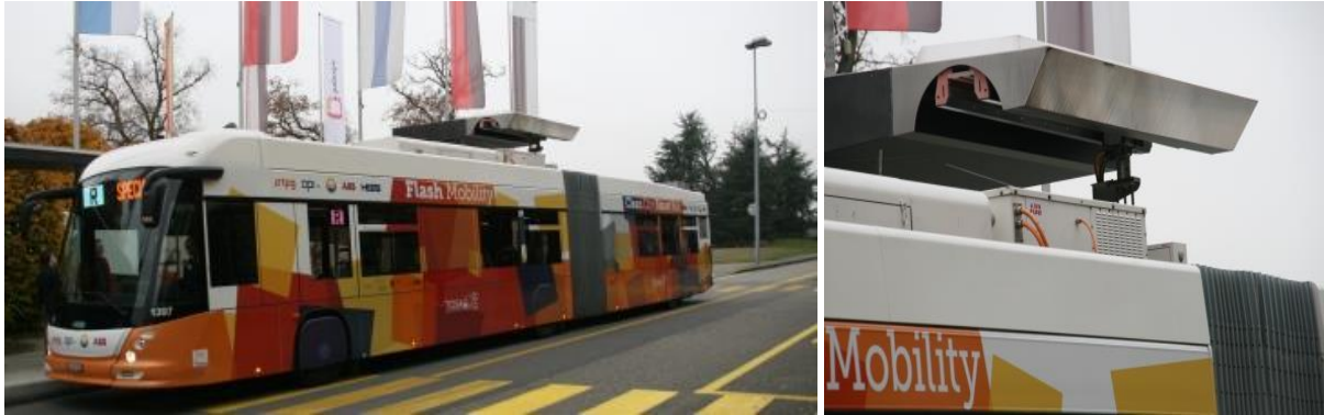
Photo 1: Flash Charging of Electric Buses (TOSA 11 )
