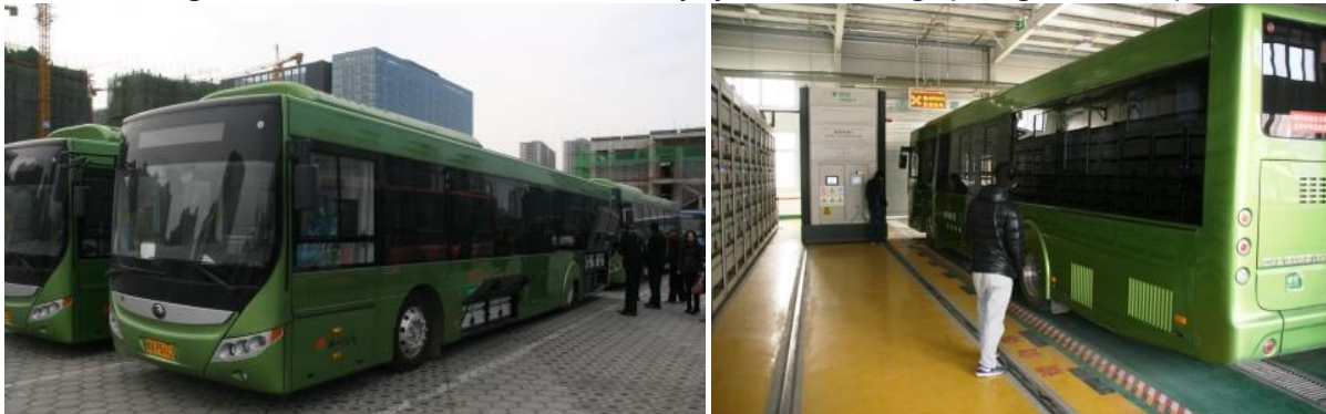
Photo 7: Yutong Electric 12m Bus and Robotized Battery System Inetrchange (Zhengzhou, China)
