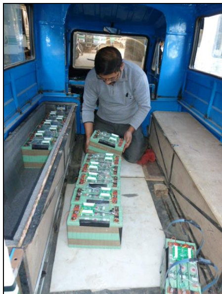
24. Mounting of batteries
