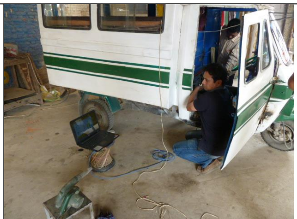
48. Technician Anil does maintenance work: checking of battery condition
