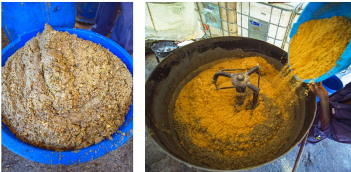
Treatment Unit, balancing different organic waste streams to create a suitable feeding substrate
