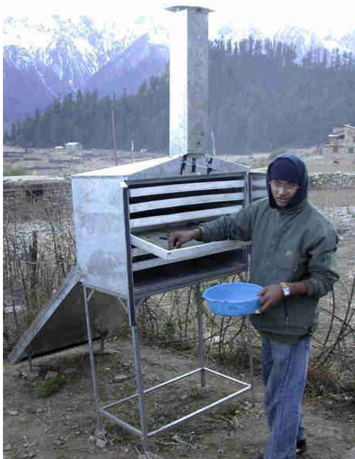
Fig. 13: RIDS-Nepal's Large, for more commercial use, solar drier in use. It can dry products (vegetables, herbs, meat etc.) in an indirect way, so that there is no discoloration, which makes it easier to sell the dried products.
