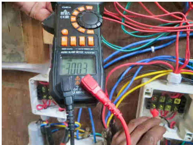
Pic. 11: RIDS-Nepal staff measuring the electricity generation of Turbine No. 2 generating 300.3 Volt DC.
