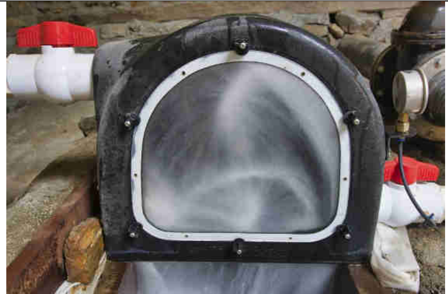
Pic 12: PowerSpout Pelton turbine running with its two jets
