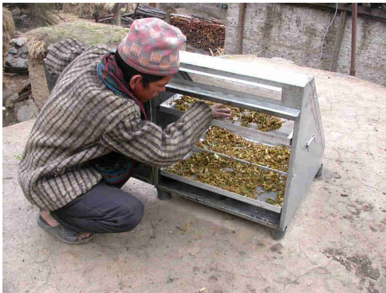
Fig. 14: The local families in Mohari village are instructed how to use the family sized solar drier to dry their vegetables grown in their high-altitude greenhouse, the herbs or even meat from their own animals. This smaller, family sized solar drier is part of the greenhouse project in order to dry vegetables in times of overproduction to store them under safe conditions for the harsh four winter months.
