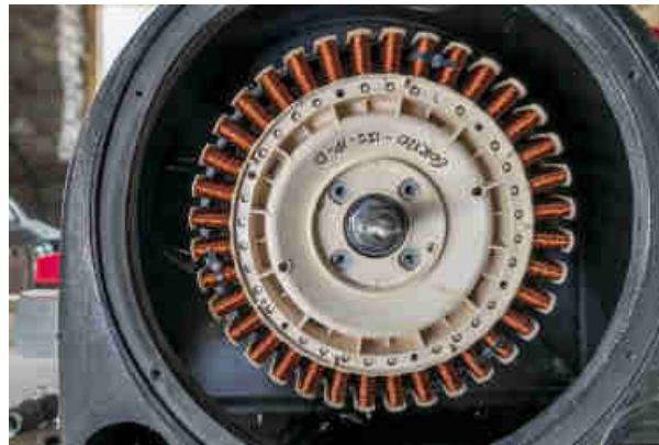
Pics 73-75. Connecting new, armoured cables to the Pelton turbines so that the cables can be put underground inside the turbine house. Each PowerSpout Pelton turbine has 48 stator fingers with a rotor with 48 permanent magnets. Each PowerSpout Pelton turbine generates at 50m head and 4 L/s water 320 Volt DC, which is sent via underground, armoured copper cables (4 x 2mm 2 size) to the 300 meter away Power House.
