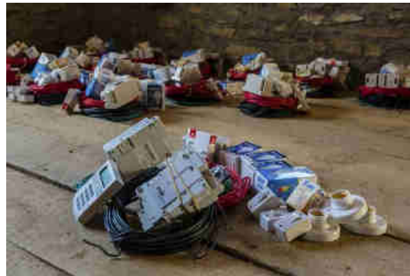
Pics. 43-45: House wiring equipment for each of the 42 homes in Mohari village. 20 m red and black cables, 4 LED lights (3 x 3watt and 1 x 5 watt), 4 bulb connectors and switches, PAYG meter, 2 Ampere MCB and insulation tape, is made available for each household to be picked up before the installation.
