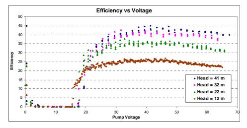
Fig 2.2. - Efficiency vs voltage for Watermax BU (Alonso-Abella [3])
