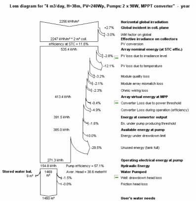
Fig 4.3. - Loss diagram for system with MPPT converter
