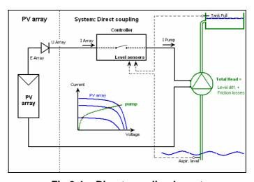
Fig 3.4. - Direct coupling layout
