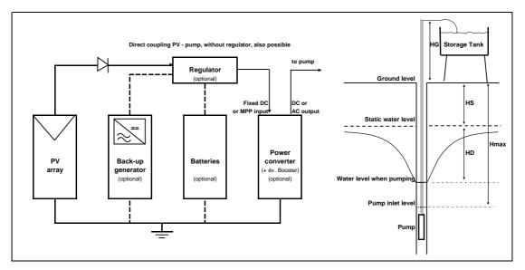
Fig 3.1. - Global schematics of a pumping system with different power conditioning / coupling options
