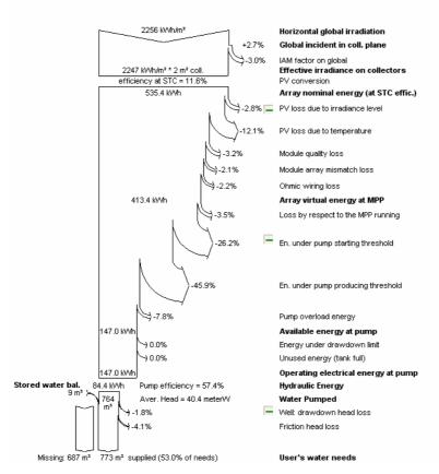
Fig 4.2. - Loss diagram for direct coupling system
