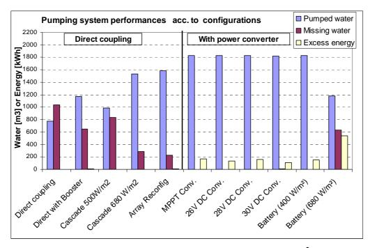
Fig 4.5. - Comparison with Water needs increased to 5 m<sup>3</sup>/day
