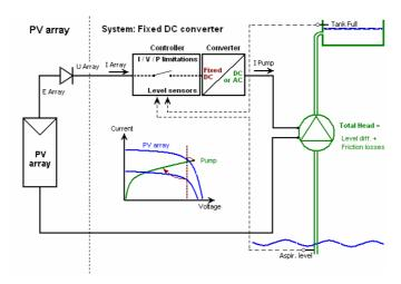
Fig 3.9. - DC-DC power converter
