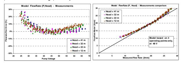
Fig 2.6. - Error with model based on only 4 points at 48V.
