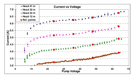
Fig 2.3. - Measured I/V data of the pump Watermax BU (Alonso-Abella 2004)
