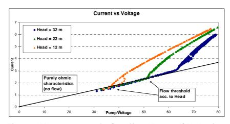
Fig 2.9. - Measurements of a Centrifugal Pump - I/V behaviour
