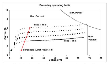
Fig 2.1. - Boundary limits of the operating domain and I/V measurements for pump Watermax BU (CIEMAT measurements [3])
