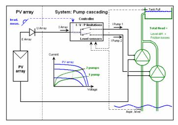
Fig 3.6. - Direct coupling with cascading
