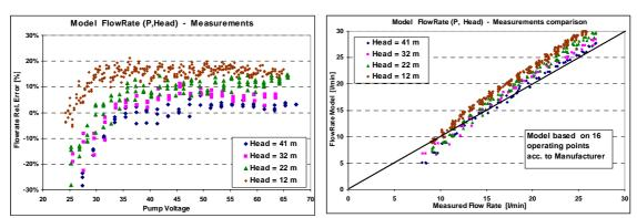
Fig 2.10. – Model – Measurement comparisons with Manufacturer's data
