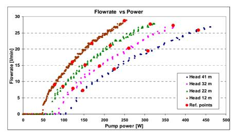
Fig 2.4. - Measured Flow/Power data of the pump Watermax BU (Alonso-Abella 2004)
