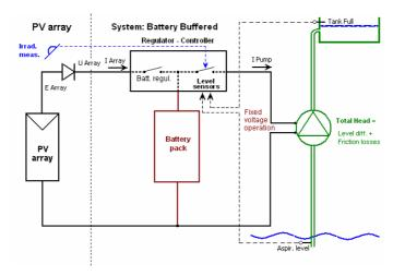
Fig 3.11. - Battery buffered system
