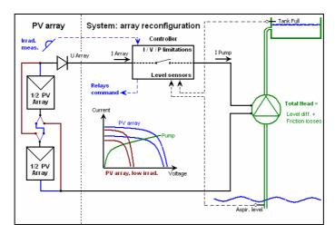
Fig 3.8. - Direct coupling with array reconfiguration
