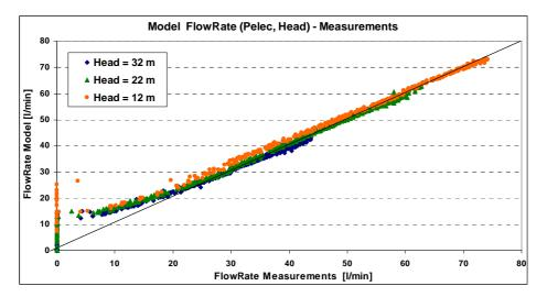
Fig 2.8. - Flowrate Model - Measurements comparison (Similarity Laws)
