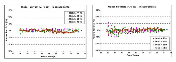
Fig 2.5. - Errors Model - Measurements, for Current and Flowrate.
