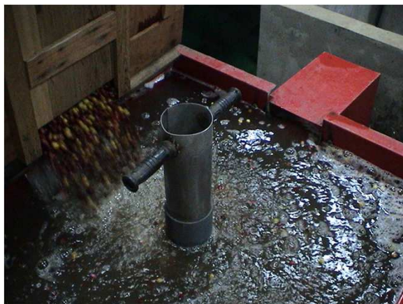
2. Sorting by Floaters (removal of fruits of bad quality)
