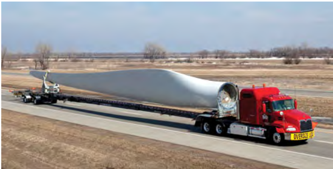
Figure 15: Extendable flat-bed trailer used to transport wind turbine blades.
