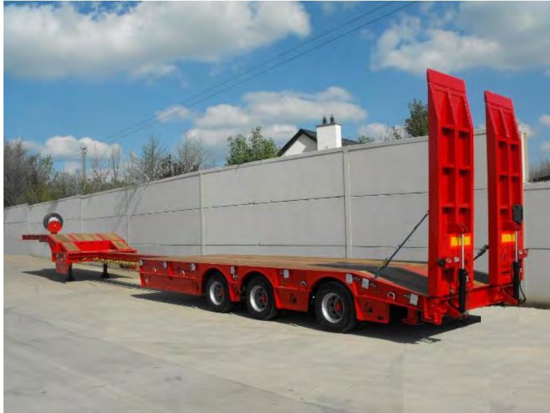
Figure 16: Three-axle trailer of the type used to transport the nacelle and hub of a wind turbine.
