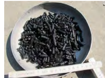
Nice biochar out of the 1.5 litres of coffee husk pellets
