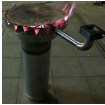
Test with prototype 2 with top blow ventilation
