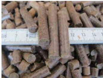
Test with pellets made out of coffee husk
