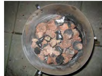
... briquettes are too big and too compact (inhibited air passage)
