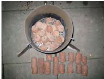
Test with coffee husk briquettes
