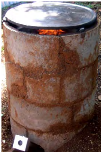
Burning injera gasifier stove prototype 3 with fan, test in Kafa
