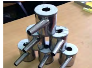
Alternative fan from Thailand, fitting the injera gasifier: cheap mass production for less than 10 dollars per piece
