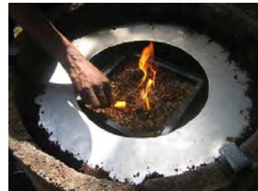
Lightening the loose coffee husk in the stove
