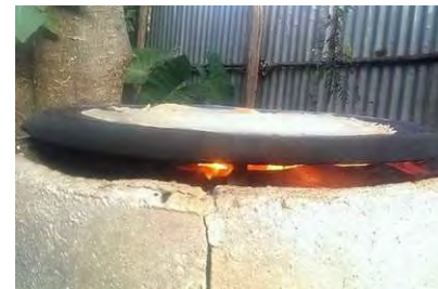
Test with baking injera – on injera gasifier prototype 3 installed through users
