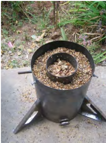
Special test with Prototype 1 in Bonga: inner cylinder with holes around is filled with wood chips, the space around is filled up with coffee husk.
