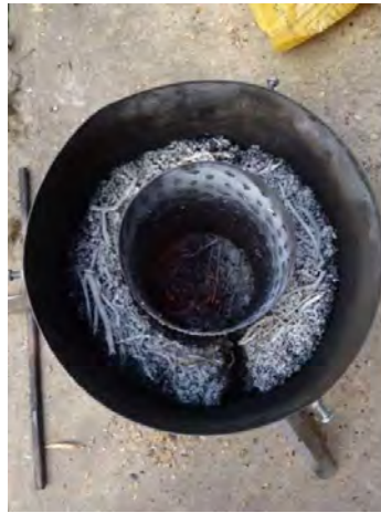
Test result: with support of one third of wood chips / wood sticks the coffee husk is carbonized easily and with a hot flame.
