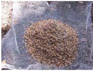
Sieving of the loose coffee husk with a mesh size of 6mm
