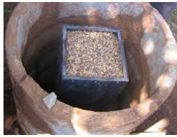
Coffee husk loaded in injera gasifier prototype 3 (rectangular shape sub-model), with the MIRT outer cylinder
