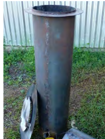
New built submodel 3 in workshop in Addis Abeba: round shaped fuel container with ventilator holder on the bottom.
