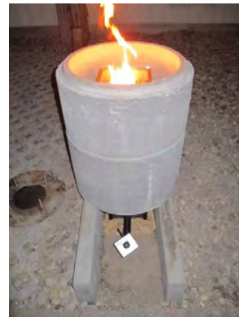
Test prototype 3: with outer cylinder made out of a concrete tube. The fan connector tube is the handle of the bio-char gate as well.
