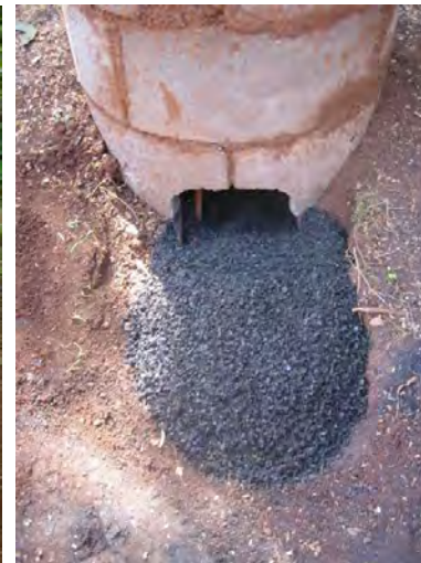
Perfectly resulted biochar out of the coffee husk
