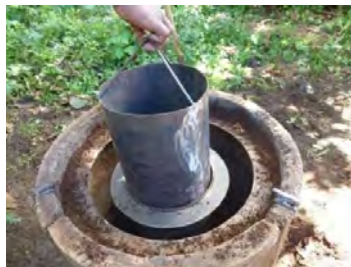
Putting the removable biochar container into the inner cylinder
