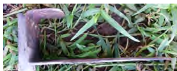
Other adapted part for fixing injera plate and burner unit with fixed gap
