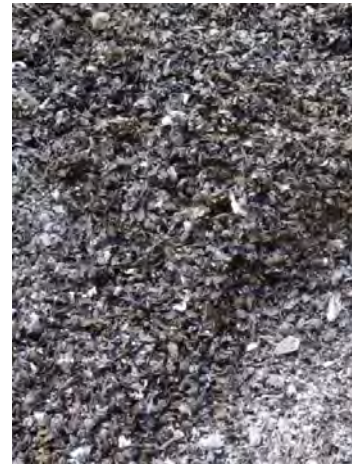
Test result: nice biochar out of coffee husk and some wood chips.
