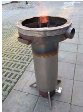
Test with bottom blow ventilation (pre-design of prototype 3).
