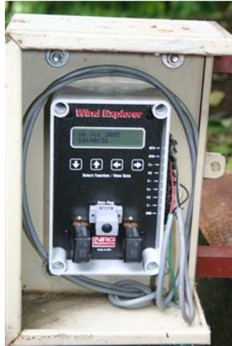
Fig. 7 The NRG data logger "Wind Explorer" used in this project
