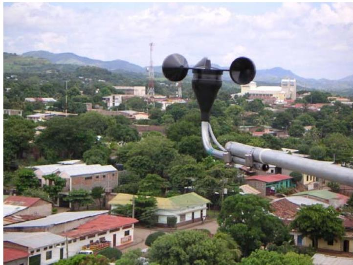
*Fig. 9 The Juigalpa site was sited in a valley that proved to have a poor average annual wind speed*
