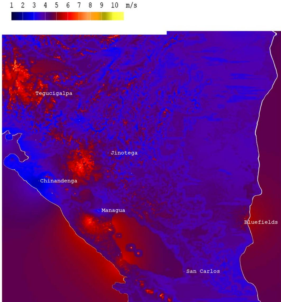
At 50 m above ground the wind speed varies between 1.0 and 8.4 m/s at 100 m between 1.2 and 9.0 m/s. The standard deviation at the measurement points is 0.9 m/s. The accuracy is about 1.5 m/s.
