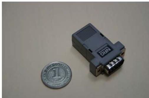
*Fig. 6 The NRG data plug can store up to six months of data*
