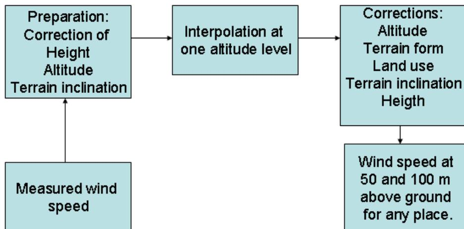
The diagram above shows the most important steps from measured wind speed to wind speed maps at 50 and 100 m above ground. Details of the procedure are given in Annex 5.
