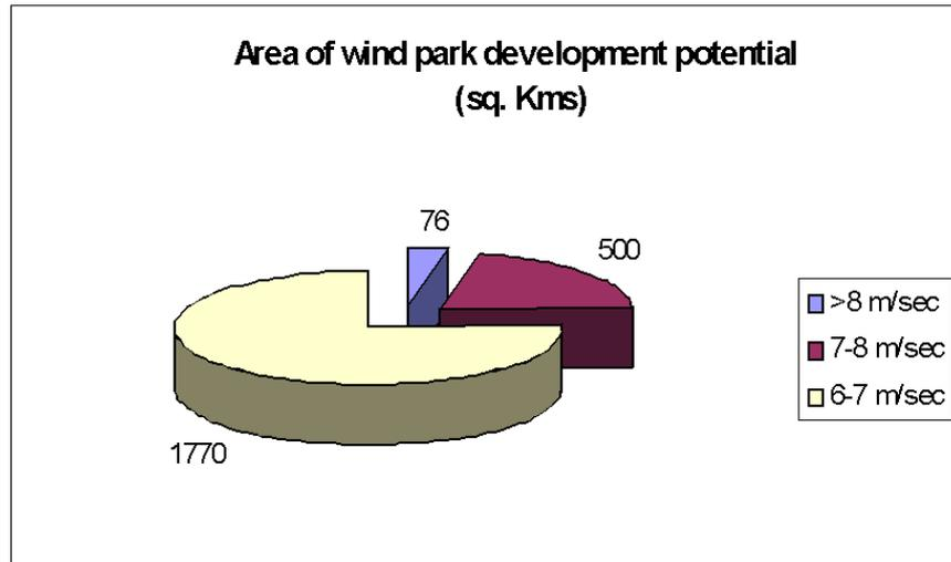
Fig. 15 Area of Wind Park Development Potential by average wind speed
