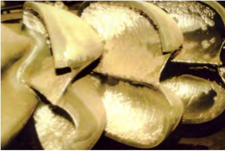
Picture 6.1 Damaged Pelton buckets caused by silt and sand
