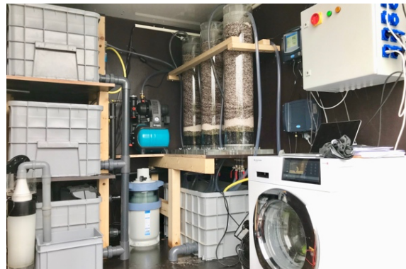
Figure 2: Interior of the LaundReCycle prototype including washing machine and installations for the water treatment
