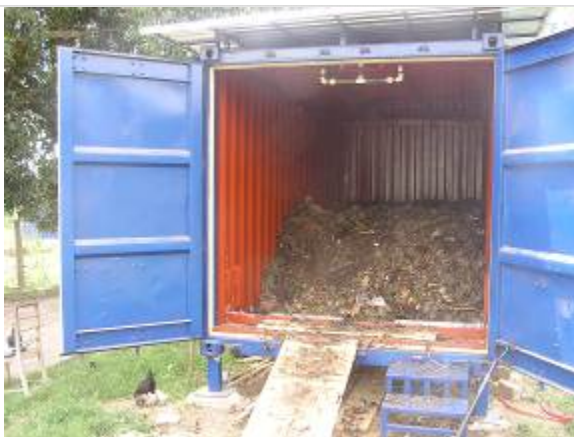
Picture 5. Filled digester
