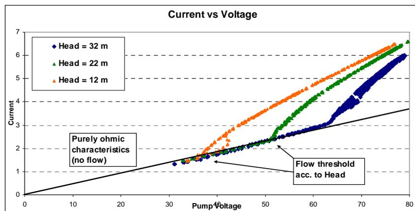
**Fig 2.9. - Measurements of a Centrifugal Pump - I/V behaviour**
