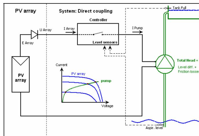
Fig 3.4. - Direct coupling layout
