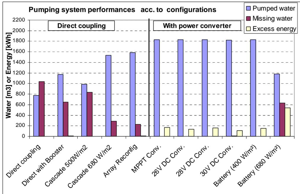
Fig 4.5. - Comparison with Water needs increased to 5 m<sup>3</sup>/day
