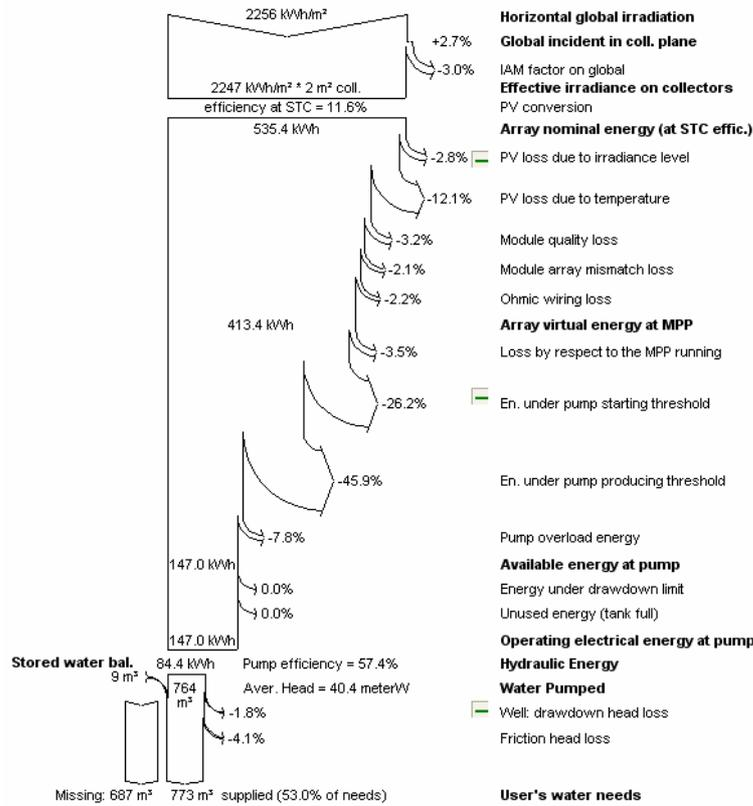
Fig 4.2. - Loss diagram for direct coupling system
