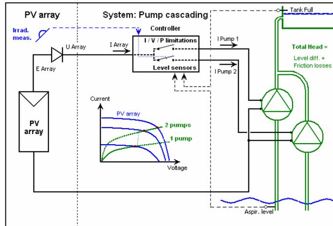
**Fig 3.6. - Direct coupling with cascading**
