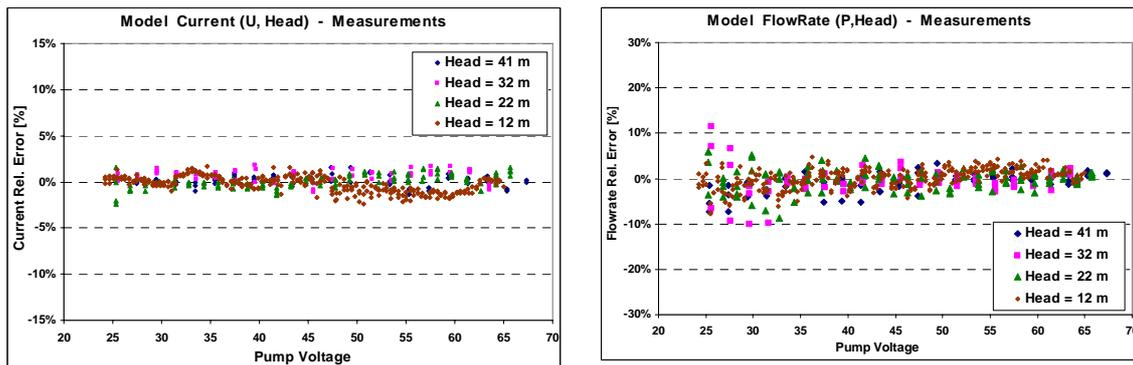
**Fig 2.5. - Errors Model – Measurements, for Current and Flowrate.**
