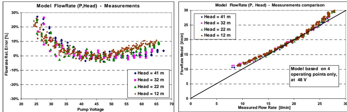
Fig 2.6. - Error with model based on only 4 points at 48V.
