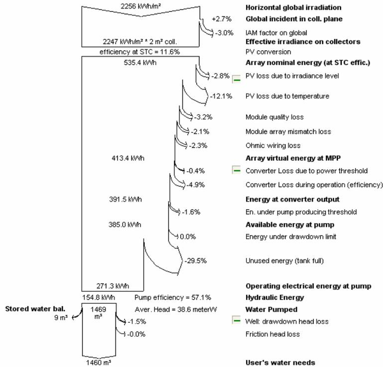
Fig 4.3. - Loss diagram for system with MPPT converter
