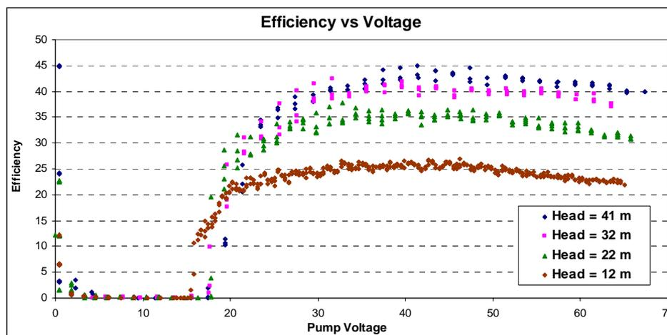
Fig 2.2. - Efficiency vs voltage for Watermax BU (Alonso-Abella [3])
