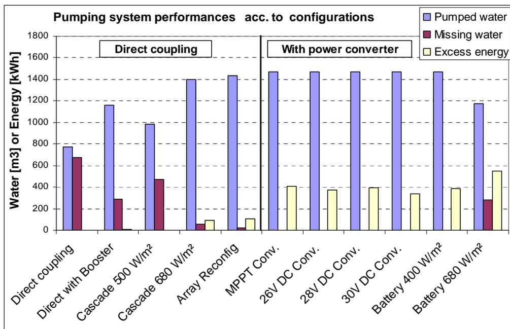
Fig 4.4. - Comparison between different system configuration performances
