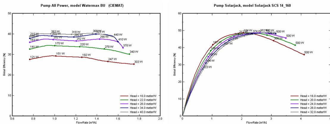
**Fig 2.11. – Example of graphs available in PVsyst. Compared efficiencies for Pos. displacement and Centrifugal pumps**
