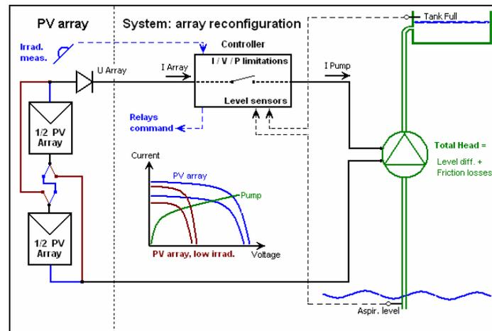
Fig 3.8. - Direct coupling with array reconfiguration
